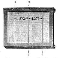
The cursor is employed whenever methods of calculation have to be employed which frequently repeat themselves and which contain constant factors, as for example the calculation of a cross section from the diameter, or the contents of a cylinder from the diameter and height. This calculation is simplified by use of the side lines which are  $1.273 = \frac{4}{\pi}$  from the centre line and results can be read off straight away, with only one setting of the cursor.
